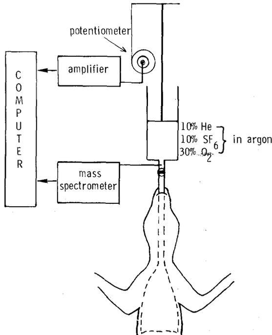
Fig. 2. Diagram of apparatus used for rebreathing measurements.
